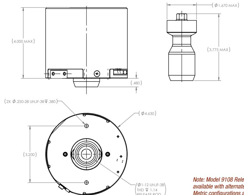
Note: Model 9108 Release Mechanism shown. Different configurations available with alternate release rods, mounting features, and connectors. Metric configurations are also available.
