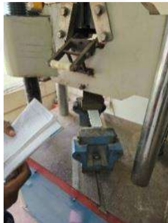
Plate 7. Flexural Test on UTM Machine
