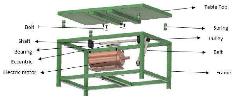
Figure 9. Exploded view of the Vibration Table
