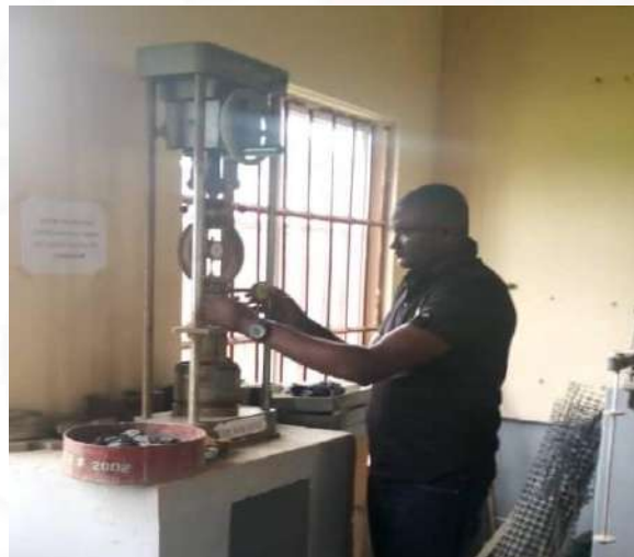
Fig. 4. California bearing ratio test setup
