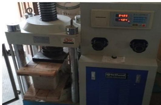
Figure 3: Compressive strength test setup
