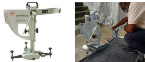
Figure 2.4: BM-III Pendulum friction coefficient tester
