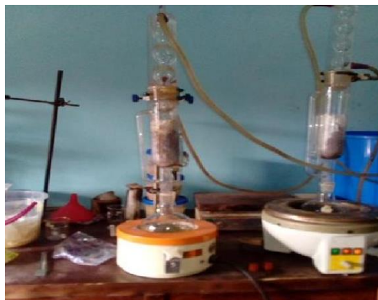
Fig. 2.1: Oil extraction using Soxhlet extractor
