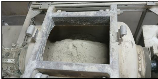
FIGURE 3: LAB CEMENT PRODUCTION IN A LAB BALL MILL
