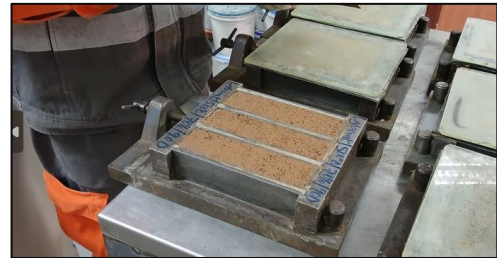
FIGURE 4: MORTAR PRISMS CASTING
