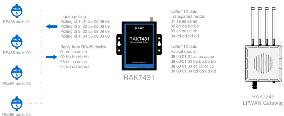
Figure 2: RAK7431 WisNode Bridge Serial polling mode
