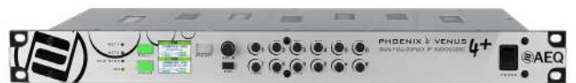
Network and communication status indicators, mains switch and mains power LED, full-colour TFT display, rotary encoder with push button and ESC cancel/return key. 12-key numeric keypad, 2 call/hang-up keys and a key to load PRESETS.
