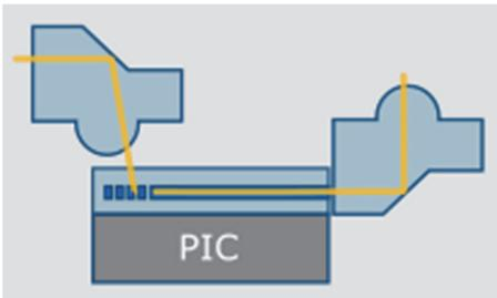
Through on-chip light guiding and manipulation Si photonics or more general photonic integrated circuits have found widespread use in data and telecom devices. Test, assembly and packaging of such devices at scale remains a challenge. Here, the combination of micro-lens and prism opens new venues enabling out-of-plane coupling using edge couplers or into-plane coupling of prism couplers.
