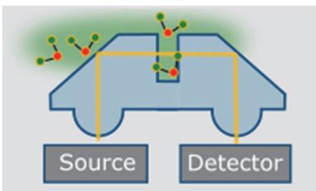
Optical principles are widely used in environmental monitoring of e.g. CO<sub>2</sub> and VOCs. Also the acquisition of healthcare data, e.g. heart rate and glucose, in consumer wearables is optics based. Providing a well-controlled and robust interaction volume for the light and the analyte of interest is paramount to good sensing performance. The microprism allows to miniaturize the transmission or evanescent field based probes known from large-scale analytic equipment.
