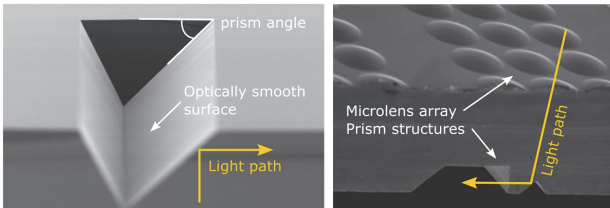
The above figures show examples of prism surfaces and microlenses structured into a Silicon substrate. Through reflection at the interface between the air and the bulk Si the light is redirected parallel to the substrate surface. The manufacturing process enables great design freedom as quantified by the guideline values in the below table:
