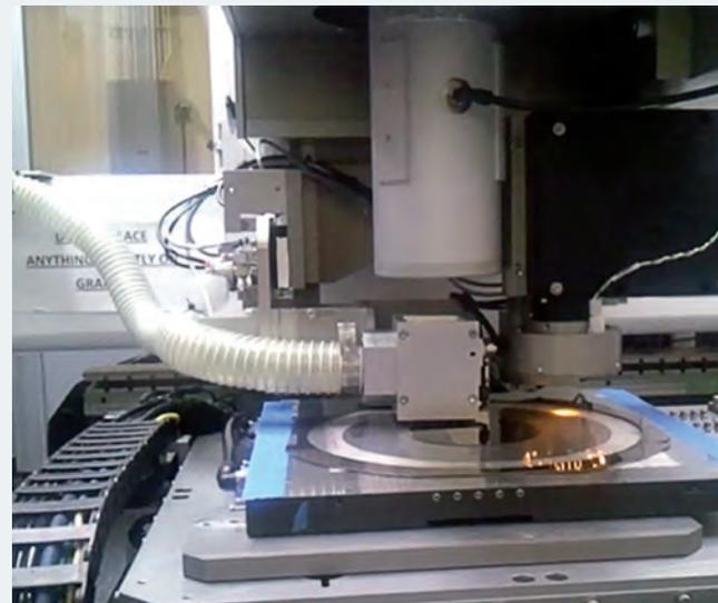
Figure 5. setup of laser de-bonding with 248 nm UV excimer laser and x-y moving stage
