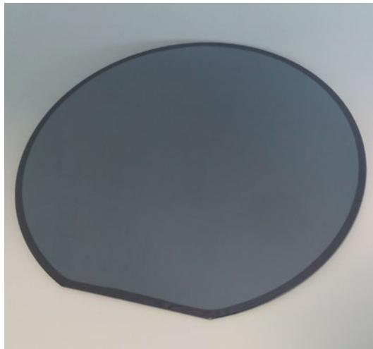
Figure 6 Wafer coated with a protection layer using contour move
