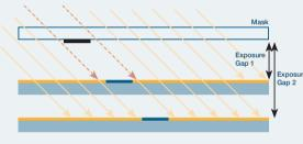
Figure 3: Schematic illustration of pattern printing shift caused by angular exposure
