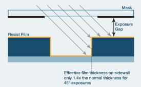
Figure 2: Angular exposure of deep trenches and vertical sidewalls
