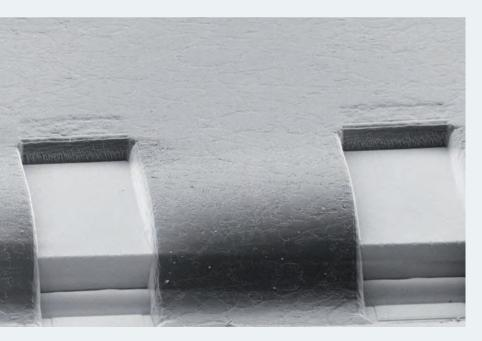
Figure 4: SEM image of spray coated, exposed and developed resist pattern for the metal interconnect
