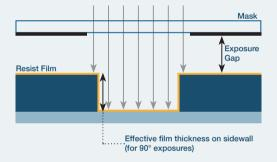
Figure 1: Standard perpendicular exposure of deep trenches and vertical sidewalls
