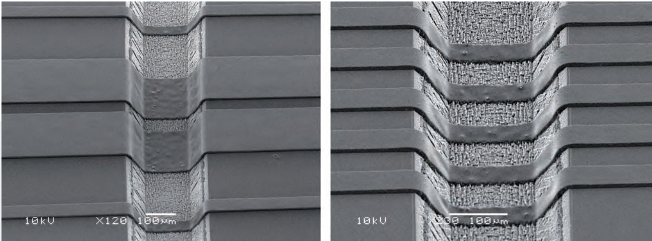
Figure 4. 50 μm and 150 μm L/S in conformal coated AZ 4999 across 200 μm deep etched trenches. Exposed on a SUSS MicroTec Mask Aligner with dedicated illumination optics.
