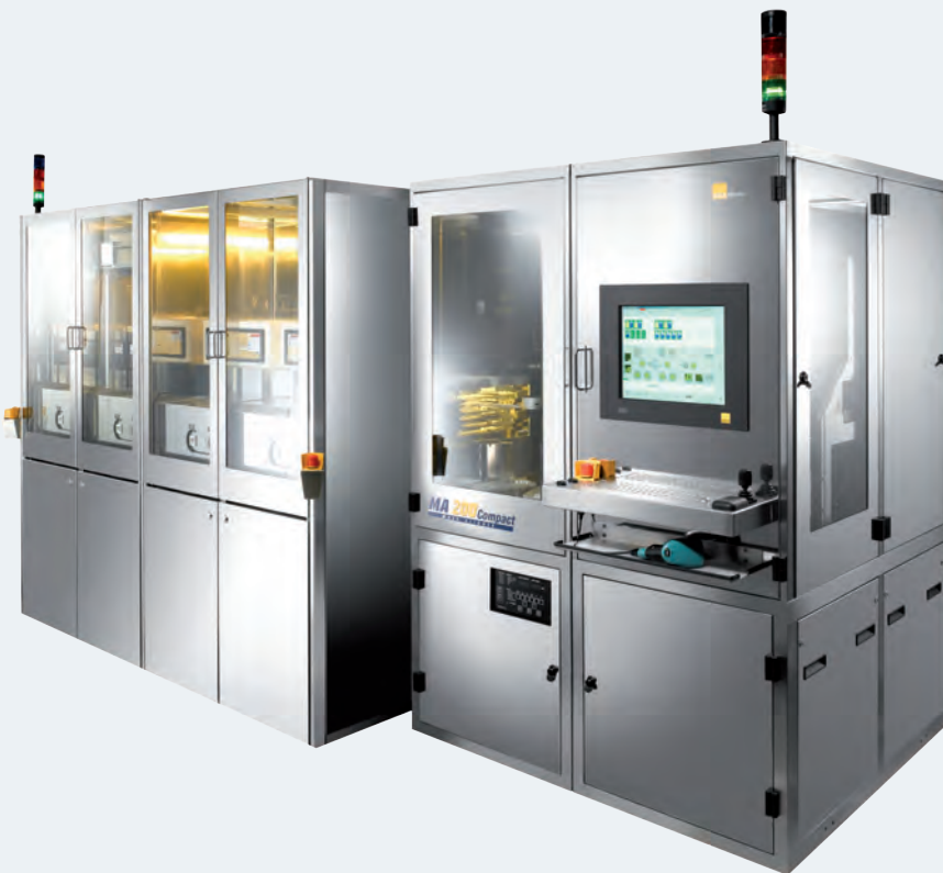
Figure 2. SUSS MicroTec LithoFab200. The fully integrated cluster for coating, baking, exposing and developing of substrates from 2" to 200mm is specifically designed for volume production.
