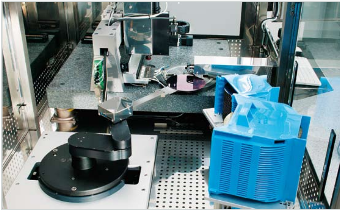
Figure 2: View of tool with robotic handling, cassettes and non- contact prealigner
