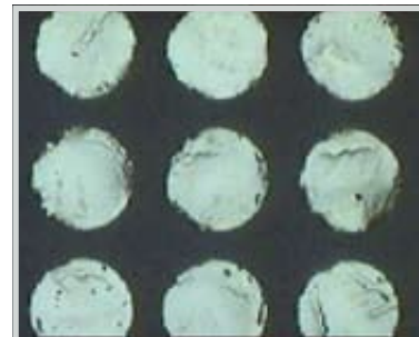
Figure 9: Filled micro-bump cavities
