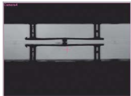
Figure 3: The ContactView system is used to assist operators in setting contact between the probe card and the wafer. Shown here is a FormFactor vertical probe card at separation and in contact. The mirrored image at the bottom of the picture is the probe card's reflection on the surface of the wafer
