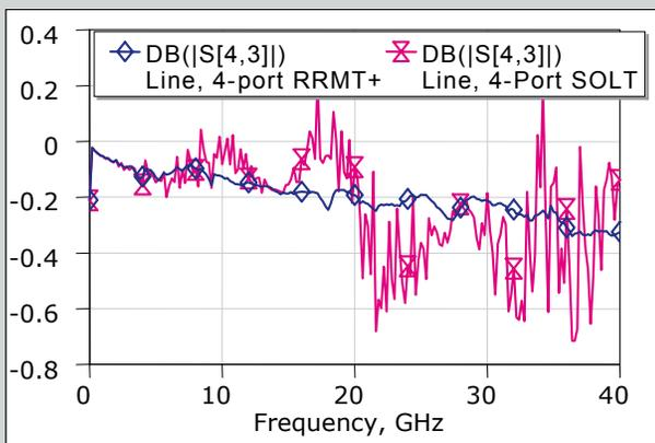
**Figure 8:** Insertion loss measurements of the dual 6000  $\mu\text{m}$  line between port 3 and port 4 with respect to the 4-port SOLT and 4-port RRMT+ calibrations.
