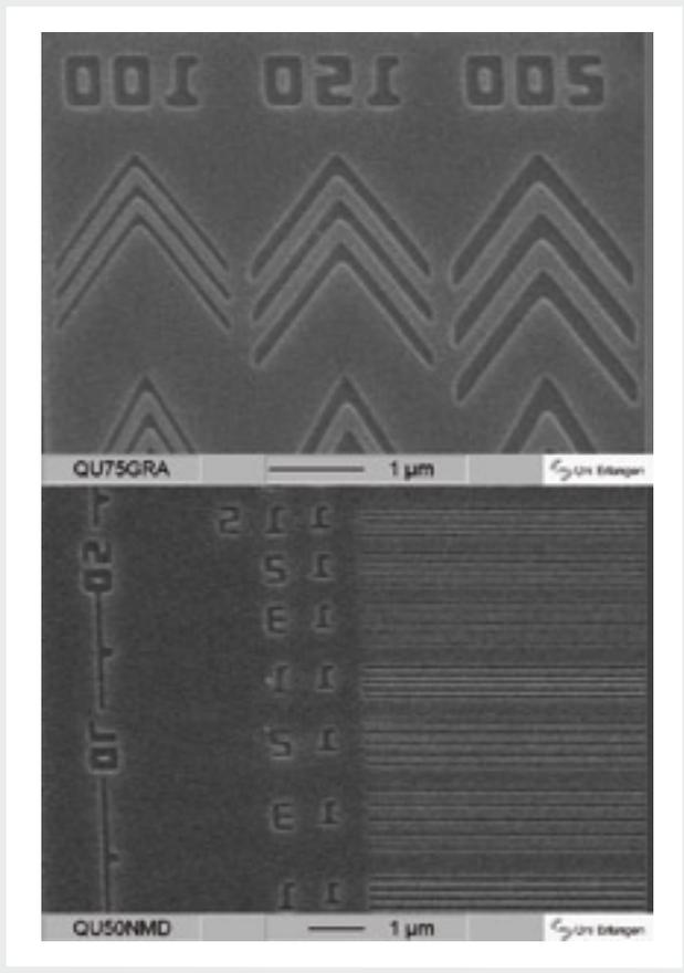
**Figure 3:** SEM images of first UV nanoimprints with the imprint tool NPS 300. On the upper image, pattern sizes from 100nm to 200nm, and on the lower image, pattern sizes from 50nm to 70nm are transferred into PAK 01.
