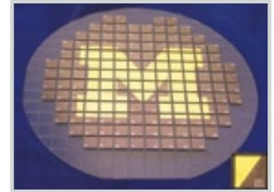
**Figure 2:** Picture of the bonded and diced lead-free flux-free solder bonded wafer.
