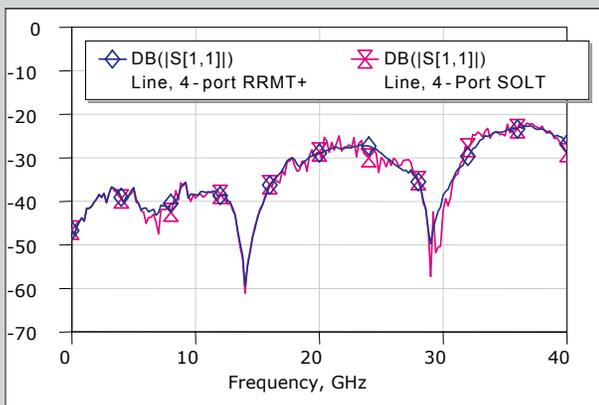
**Figure 7:** Return loss measurements of the dual 6000  $\mu\text{m}$  line on port 1 with respect to the 4-port SOLT and 4-port RRMT+ calibrations.
