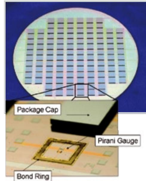
**Figure 7:** Picture of a 4" wafer with nickel-tin diffusion soldered packages. The bottom picture shows an intentionally decapped package with the bond ring and Pirani gauge inside.
