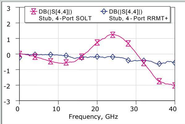
**Figure 6:** Return loss measurements of the dual 6000  $\mu\text{m}$  stub line on port 4 with respect to the 4-port SOLT and 4-port RRMT+ calibrations.
