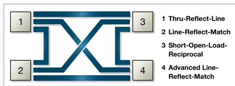
Figure 1: Configuration of thru standards for a 4-port wafer-level calibration: straight thru (port 1 – port 2, port 3 – port 4), loop-back thru (port 1 – port 3, port 2 – port 4), cross-over thru (port 1 – port 4, port 2 – port 3).
