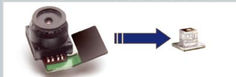
Figure 1 On the left: Camera module made by using traditional semiconductor and packaging technology. On the right: A camera module made using 3D interconnect technology. [Source Tessera]
