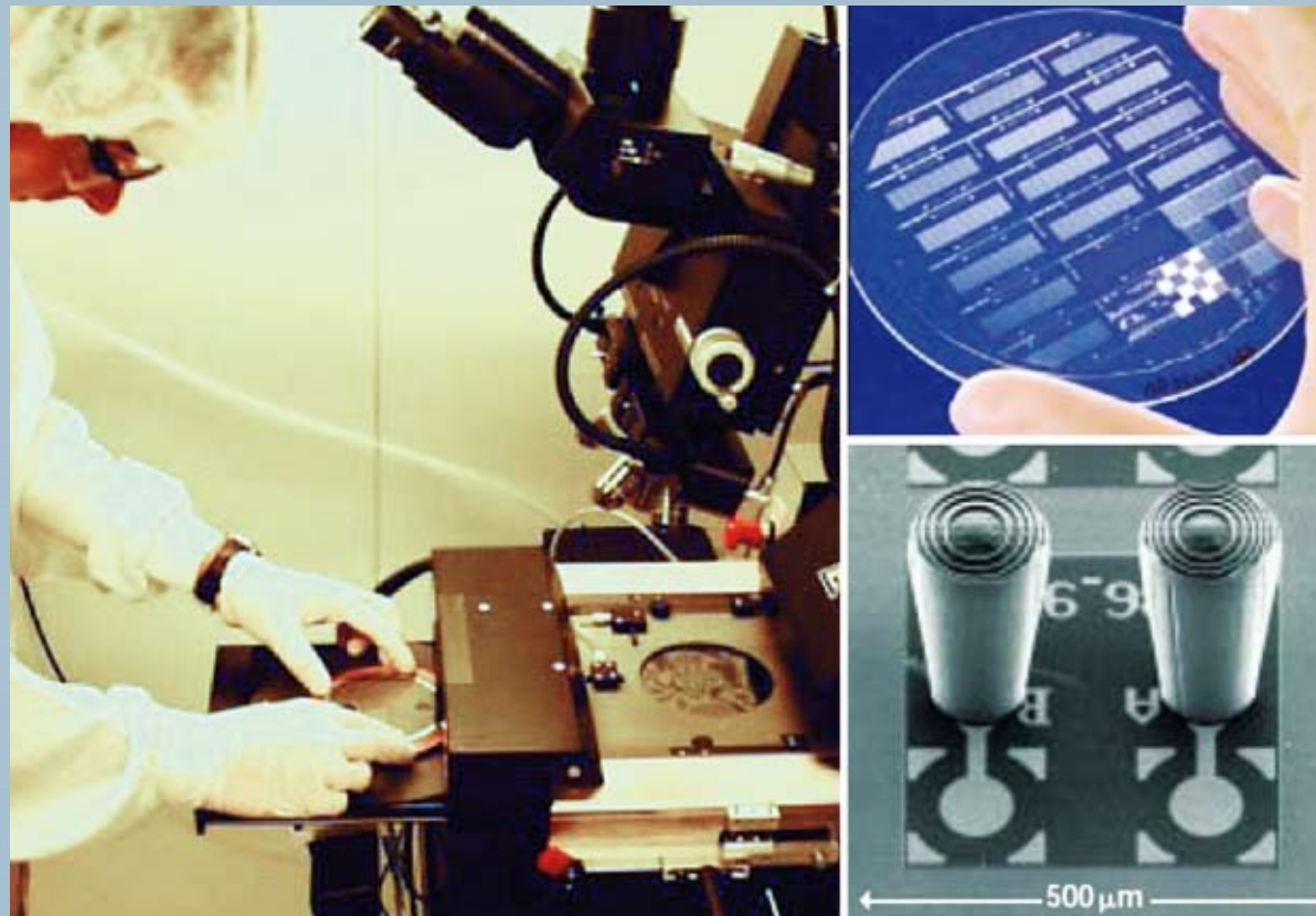
UV-embossed micro-optics using a SUSS MicroTec Mask Aligner. Sol-gel microlenses for collimation were imprinted on top of VCSELs. (Photos: CSEM Zurich)
