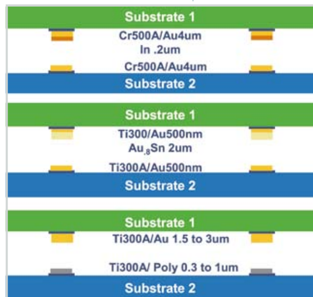
Figure 4: Typical seed layer and eutectic/metal stack thicknesses for (a) AuIn, (b) AuSn and (c) AuSi eutectic bond seal rings for MEMS wafer bonding
