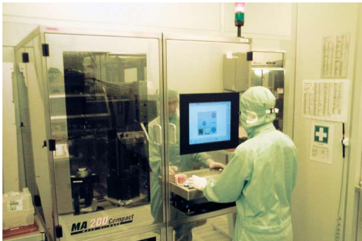
Figure 7: Double side lithography for cap wafer processing is performed with a SUSS MA200 Compact
