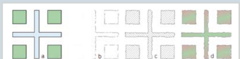
Figure 5: schematic drawing of polymeric alignment marks and their microscope images. a) mark as designed, b) left half: very weak contrast as obtained with standard reflected light illumination, right half: stronger contrast with transmitted light. Still the pattern is not ideally suited for pattern recognition due to its narrow contrasted structures. c) internal surface patterning of the target to enhance contrast and create expanded structures d) contrast as obtained with DIC microscopy or similar method resulting in better contrasts and expanded structures
