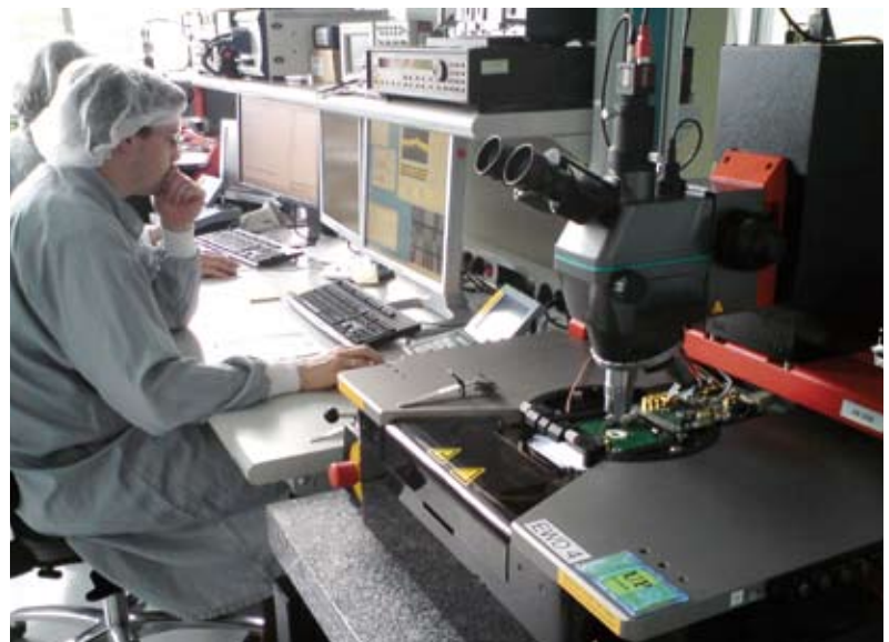
Figure 6: SUSS PA200 MEMS wafer probers are used for sensor characterization and leak test by Q-factor monitoring
