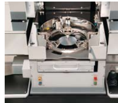
Photo 7: The MA/BA8 Gen3 can be configured as mask and bond aligner combination or as bond aligner only.
