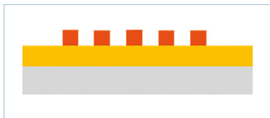
Figure 2 Conductors patterned with photoresist which is stripped after patterning
