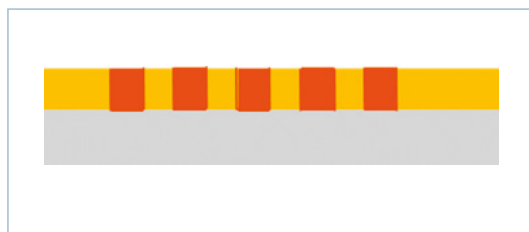
Figure 3 Conductors embedded in polyimide
