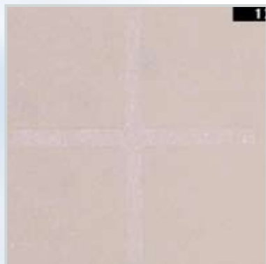
Figure 1: Microscope image of an alignment target on a GaN-Wafer. The contrast between the target cross and the background is very poor.
