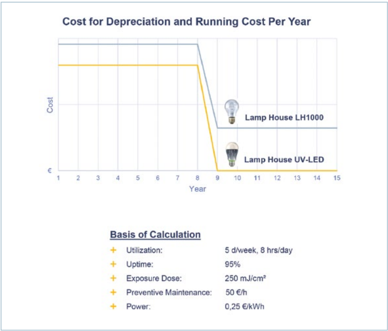
Figure 4 Comparison of cost between Hg lamp house and UV-LED lamp house
