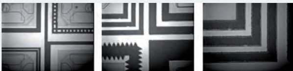
Figure 7. Transmission IR images) from an offline IR microscope at 50, 100 and 200x magnification shows seal-rings from aligned and bonded AlGe substrates
