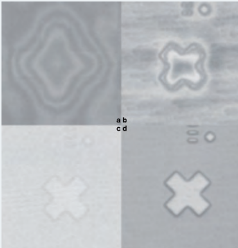
Figure 2. Influence of illumination on target visibility. Microscopic images acquired with different illumination settings. a) undefined customer illumination, b) red LED, c) yellow filtered white LED (6000K), d) yellow filtered white light halogen (3200K)
