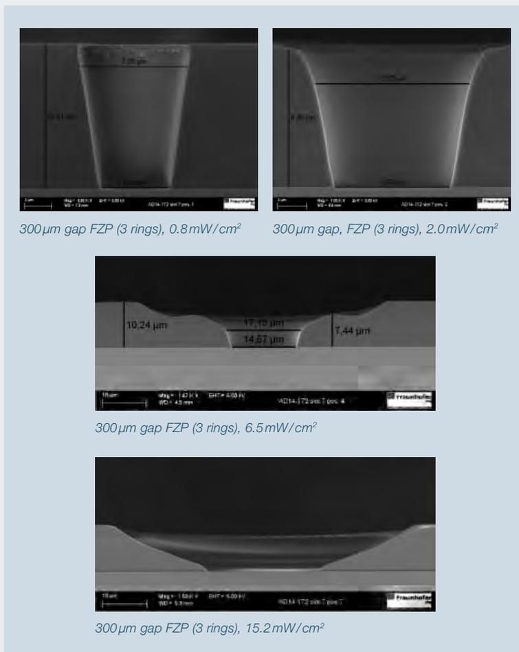
Figure 5 SEM images for  $10\mu\text{m}$  thick AZ9260 at  $300\mu\text{m}$  proximity gap, 40s exposure time,  $300\mu\text{m}$  gap FZP design (3 rings)
