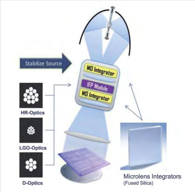
Figure 5 Conceptual drawing of SUSS MO Exposure Optics with exchangeable illumination filter plates
