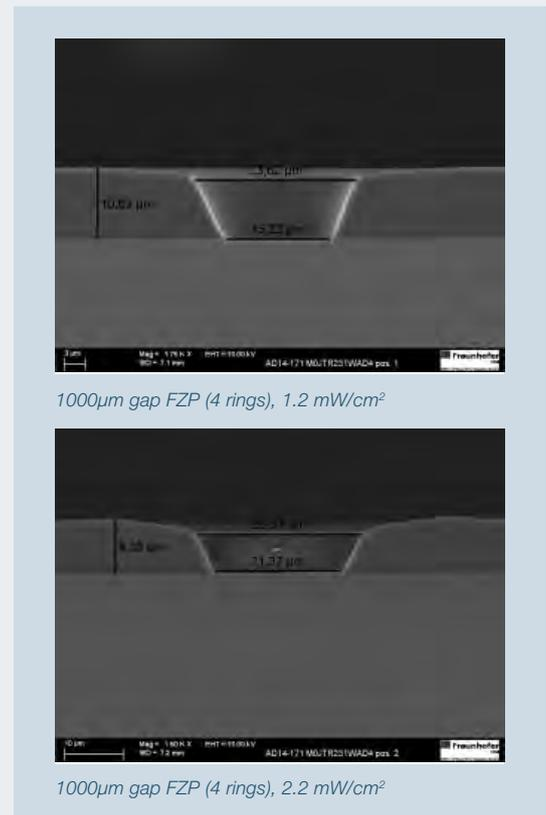
**Figure 7** SEM images for 10 $\mu\text{m}$  thick AZ9260 at 1000 $\mu\text{m}$  proximity gap, 60s exposure time, 1000 $\mu\text{m}$  gap FZP design (4 rings)
