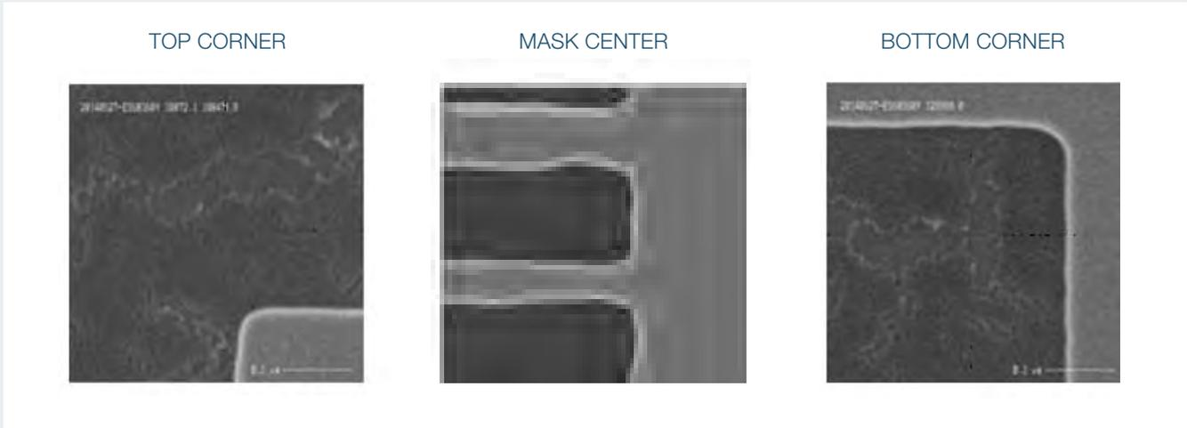
**Figure 5** SEM image of Chemical A treated EUV test pattern: Ruthenium capping layer peeling-off was observed in the top and bottom mask corners (left and right images). No damage was observed for the central region of the EUV mask
