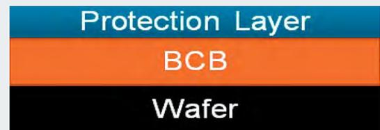
Figure 6 Principle of a protection layer for laser ablation
