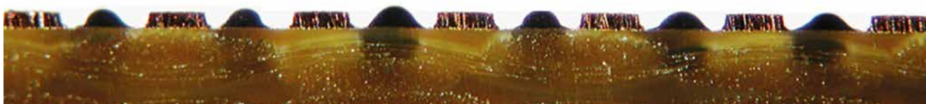
The cross sections in this page show a typical inkjet solder mask profile. Accurate thickness design at copper edge and well positioned dams between pads enable high functional reliability for PCB manufacturing.
