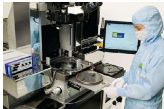
Figure 1: The MA8 Gen3 supports photolithography, UV bonding, UV replication bond alignment and NIL
