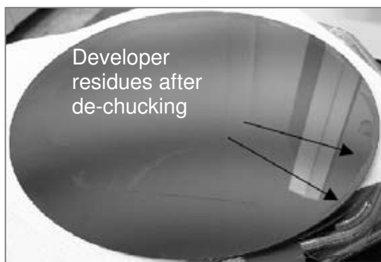
Figure 6: Standard T-ESC carriers should not be used in the lithography process because wet chemicals (e.g. developer) are pulled between carrier and wafer.
