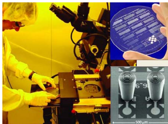
Fig. 3. UV-embossed micro-optics using a SUSS Mask Aligner. Sol-gel microlenses for collimation are imprinted on top of VCSELs (photos CSEM Zurich).
