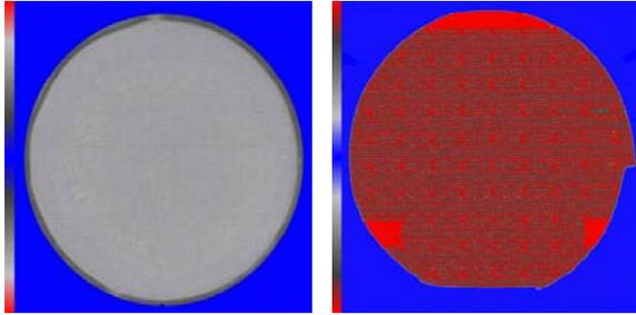
**Figure 9. Left is a blanket layer of aluminum on a 200mm wafer successfully bonding with Al diffusion techniques. On the right is a 150mm device wafer also bonded with aligned Al to Al diffusion methods.**
