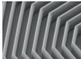
Wafer Level Packaging Structure of a RFID transponder chip as used for ID tags or electronic toll collection systems. 30 μm negative JSR THB 126N resist Courtesy: FhG IZM
