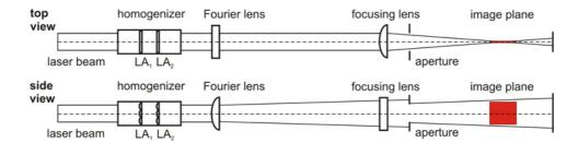
Figure 1. Optical set-up of the experiment.
