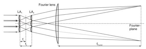
Figure 2. Schematic principle of beam homogenization.
