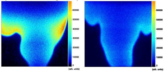
Figure 5: single-shot OH-LIF images *without* the application of the beam homogenizer (left) and *with* the homogenizer (right) resulting in the desired homogeneous "flat-top" beam profile
