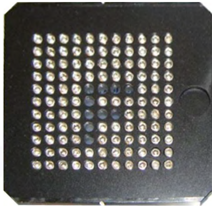
Simple pattern change with pixelated Illumination Filter Plate (IFP)
