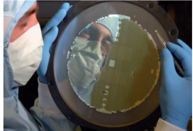
Figure 37 An 8" wafer with VGA lenses on blue tape after dicing. The wafer-level cameras (WLCs) consist of two wafers with micro-optics (double-sided) manufactured by wafer-scale imprint technology and wafer-level packaging (Photo: Heptagon).
