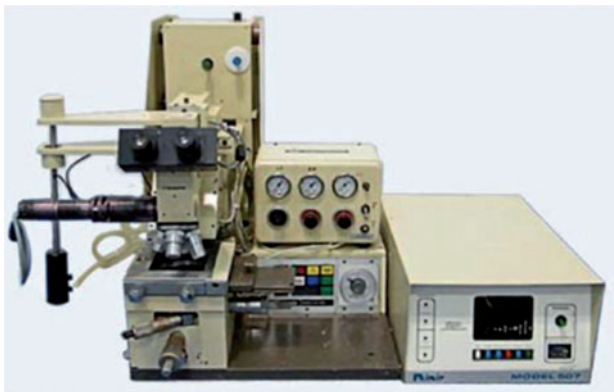
Figure 8 Karl Süss MJB3 manual contact mask aligner (Photo: SUSS MicroTec).
