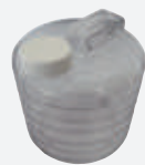
Water receiver for Water distiller
