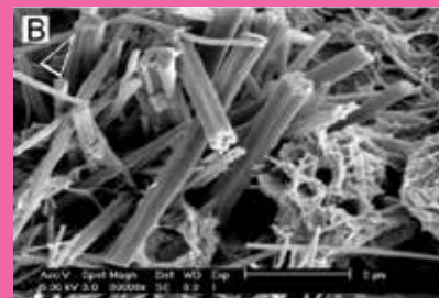
High magnification image of the calcium phosphate crystals 4 .
