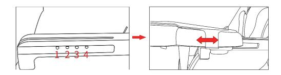
6.In order to wash the tray, you may remove its cover plate by releasing its two catches and three blocks.
