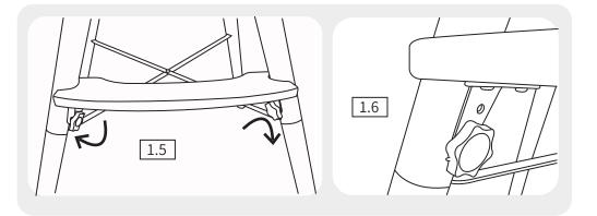
4.Assemble Tray:Position the tray over the armrest, holding the latch mechanism at both sides of the tray, at the same time sliding the tray onto the chair with the desired position, the release the latch and move the tray until a click sound is heard.
