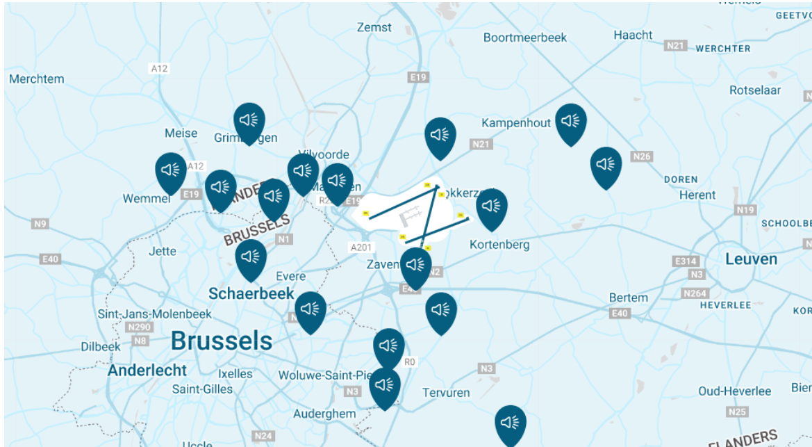
Figure 5: Network of noise monitoring terminals around Brussels airport (Source: https://www.batc.be/fr/bruit/mesures-sonores )
