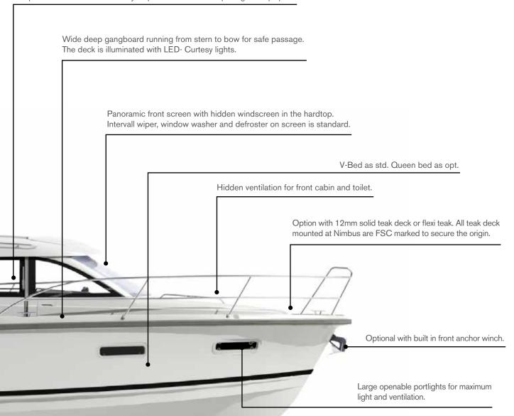
The complete boat is produced with the most modern vacuum infusion technic, The Hull, deck and the bulkhead are all vacuum infused with a core of divinycell.
