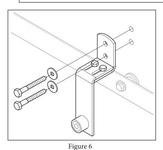
9. Install bypass brackets with a socket wrench and 9/16" socket, using lag screws and washers (provided) in the top two holes above the rail (Figure 6). Take care to not overtighten to avoid damaging the wall and stud.
