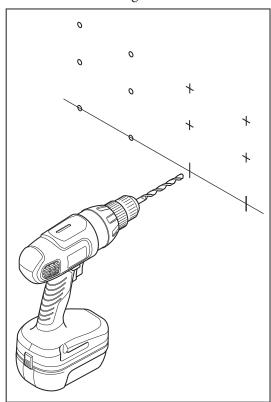
7. Drill out the marked holes using a drill with a 1/4" drill bit (Figure 4).
