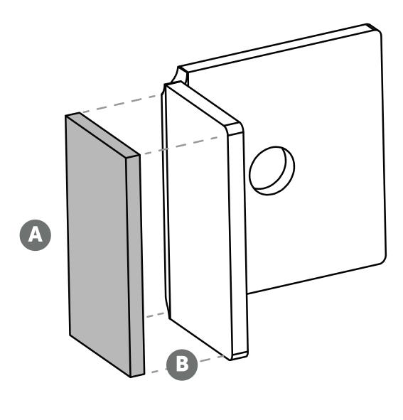
• Remove adhesive strip backing from rubber pad.
