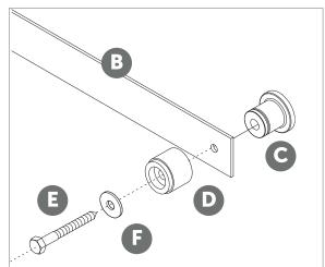
Attach one end of the track to the wall with C one spacer, O one soft stop, C one lag screw, and C one washer (provided) using a socket wrench with 9/16" socket. Do not tighten. Repeat for the other end of the track.
