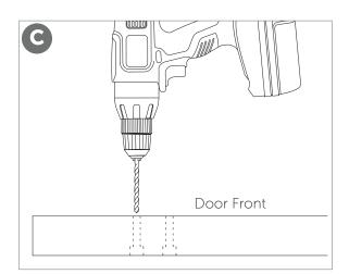
Install the hangers to the front of the door using lag bolts, washers, and acorn nuts (provided).
