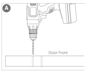
B Door Back Orill two pilot holes all the way through the door for each hanger using a drill with an 1/8" drill door for each hanger using a drill with an 1/8" drill bit.
