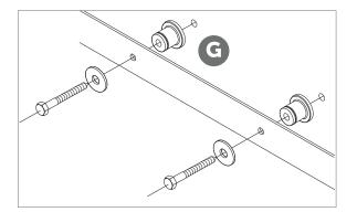
Install remaining spacers with lag screws and washers (provided) using a 9/16" socket wrench. Tighten all lag screws.
