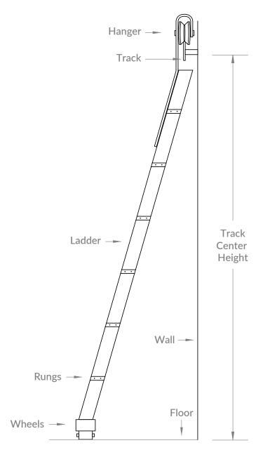
The "Track Center Height" is the distance from the floor to the center of the track. This would be where the lag bolts would attach the track to the wall. This Track Center Height helps us determine how to properly manufacture your ladder to work perfectly for the height you need to achieve for your ladder to work as it will be angled once installed.
