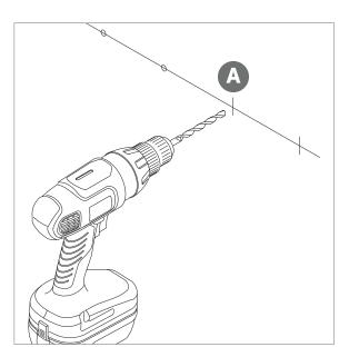
• Drill out the marked holes using a drill with a 1/4" drill bit.
