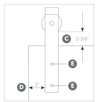
• Adjust the placement of the hanger for a 2-3/8" gap between the top of the door and the bottom edge of the wheel.
