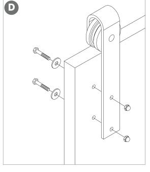
Install the hangers to the front of the door using lag bolts, washers, and acorn nuts (provided).
