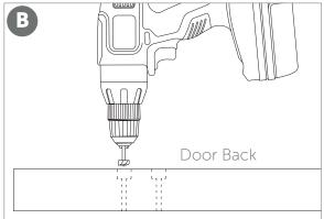
$\blacksquare$  Turn the door over. Using a 1-1/8" Forstner bit\*, drill a 7/16" deep hole into each pilot hole.
