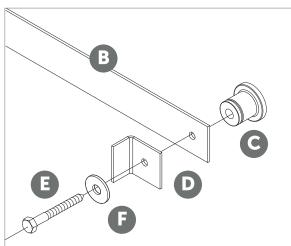
**B** Attach one end of the track to the wall with **G** a spacer, **D** one hard stop, **G** one lag screw, and **G** one washer (provided) using a socket wrench with 9/16″ socket. Do not tighten.
