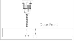
• Install the hangers to the front of the door using lag bolts, washers, and acorn nuts (provided).
