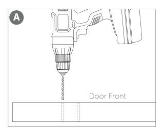
Drill two pilot holes all the way through the door for each hanger using a drill with an 1/8" drill door for each hanger using a drill with an 1/8" drill bit.
