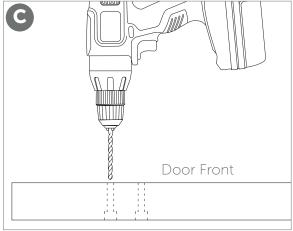
© Turn the door over, returning it to the face-up position. Drill all the way through the pilot holes using a drill with a 3/8" drill bit.
