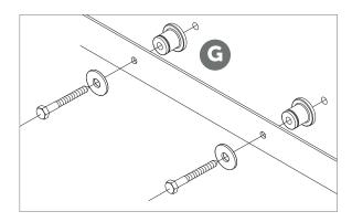
• Install remaining spacers with lag screws and washers (provided) using a 9/16" socket wrench. Tighten all lag screws.
