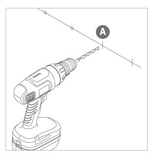
• Drill out the marked holes using a drill with a 1/4" drill bit.
