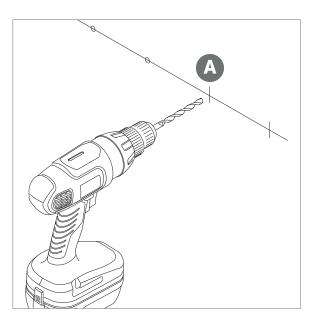
$\bullet$  Drill out the marked holes using a drill with a 1/4" drill bit.
