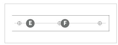
• Hold the track up to where the pencil line is visible through the holes in the track.
