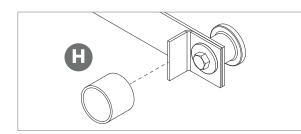
• Stretch rubber bumper (provided) over hard stop. Repeat for the hard stop on the other end of the track.
