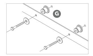
G Install remaining spacers with lag screws and washers (provided) using a 9/16" socket wrench. Tighten all lag screws.
