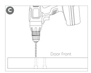
• Turn the door over, returning it to the face-up position. Drill all the way through the pilot holes using a drill with a 3/8" drill bit.
