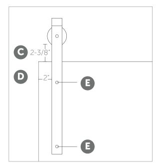
**G** Adjust the placement of the hanger for a 2-3/8" gap between the top of the door and the bottom edge of the wheel.
