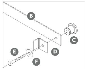
Attach one end of the track to the wall with G a spacer, O one hard stop, O one lag screw, and O one washer (provided) using a socket wrench with 9/16" socket. Do not tighten.
