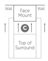
Finish by screwing in the supplied grabber screws through the pre-drilled holes in your surrounds to secure them to the face mounts. Repeat for the face mounts installed along the floor.
