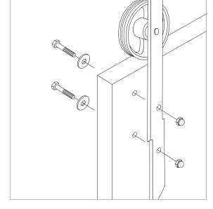
Install the hangers to the front of the door using lag bolts, washers, and acorn nuts (provided).
