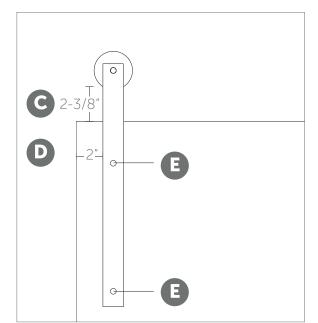
• Adjust the placement of the hanger for a 2-3/8" gap between the top of the door and the bottom edge of the wheel.
