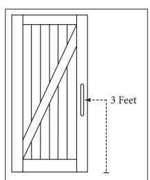
The center point of the door pull should be three feet above the bottom edge of the door. Avoid placing the door pull too close to the edge of the door. Placing the pull too close to the edge can damage both door and pull.
