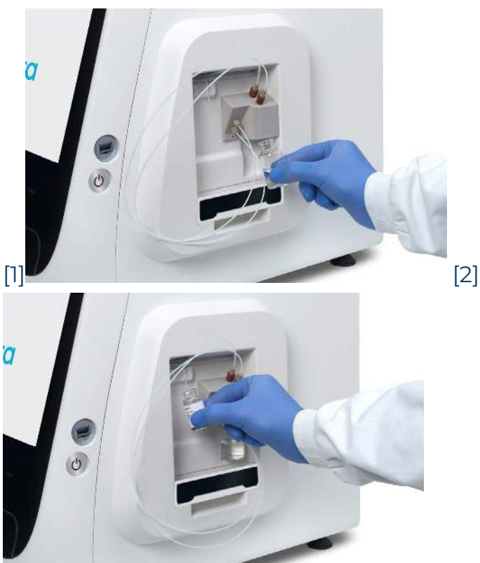
Figure 4: Connection of the empty waste container [1] and the vial of base fluid [2] to the pump
