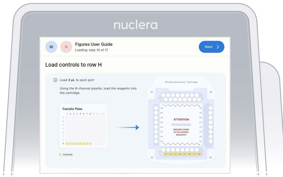
Figure 21: Loading of the reagents onto row H of the cartridge
