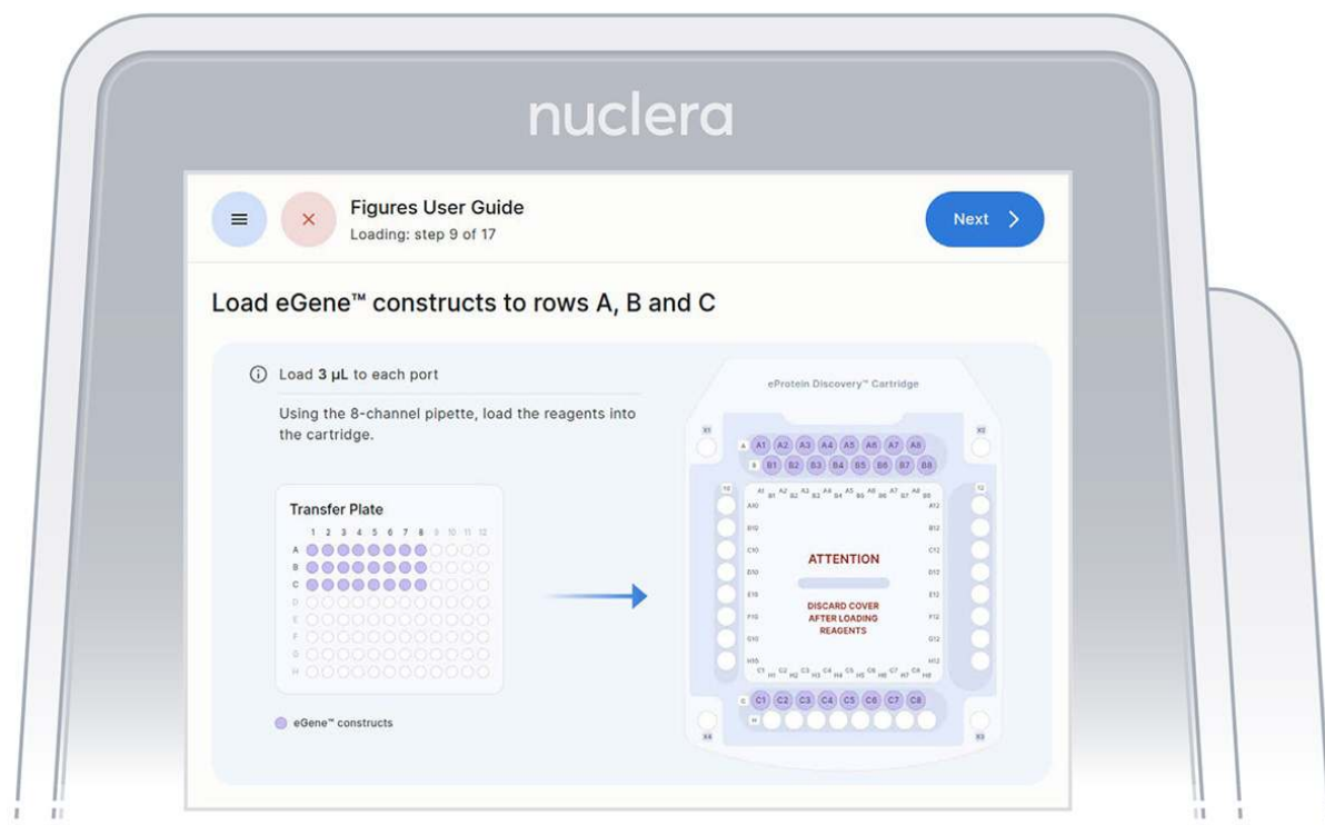
Figure 20: Loading of the eGene constructs onto row A, B and C of the cartridge
