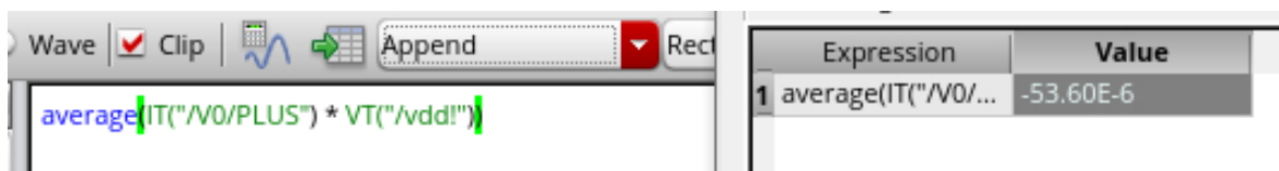
Figure 13: Power consumption of the adder - note the negative sign indicates a power draw.
