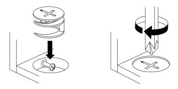
Turn cam lock clockwise to tighten.
